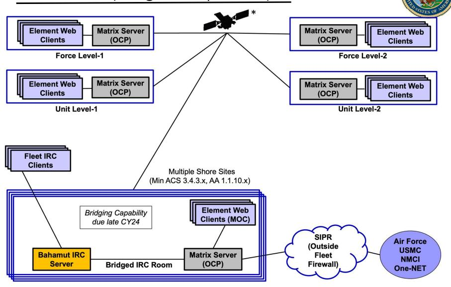
$<sup>\</sup>ensuremath{^*}$  - Note while SATCOM is shown any TCP/IP networking path can be used
